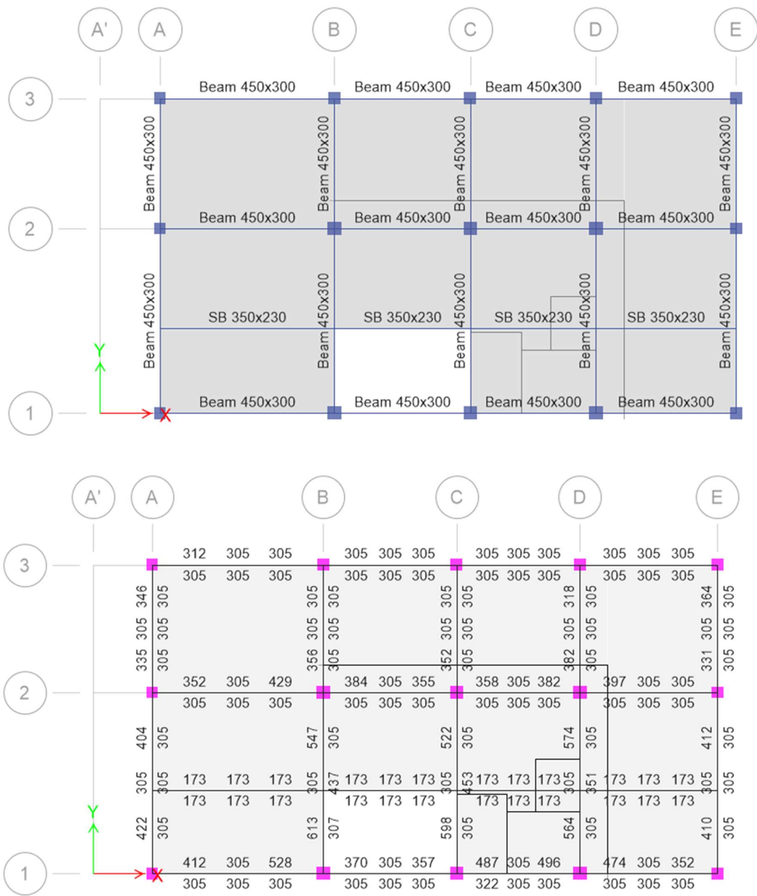
Figure 4-7: Beam sections and reinforcement at RF
