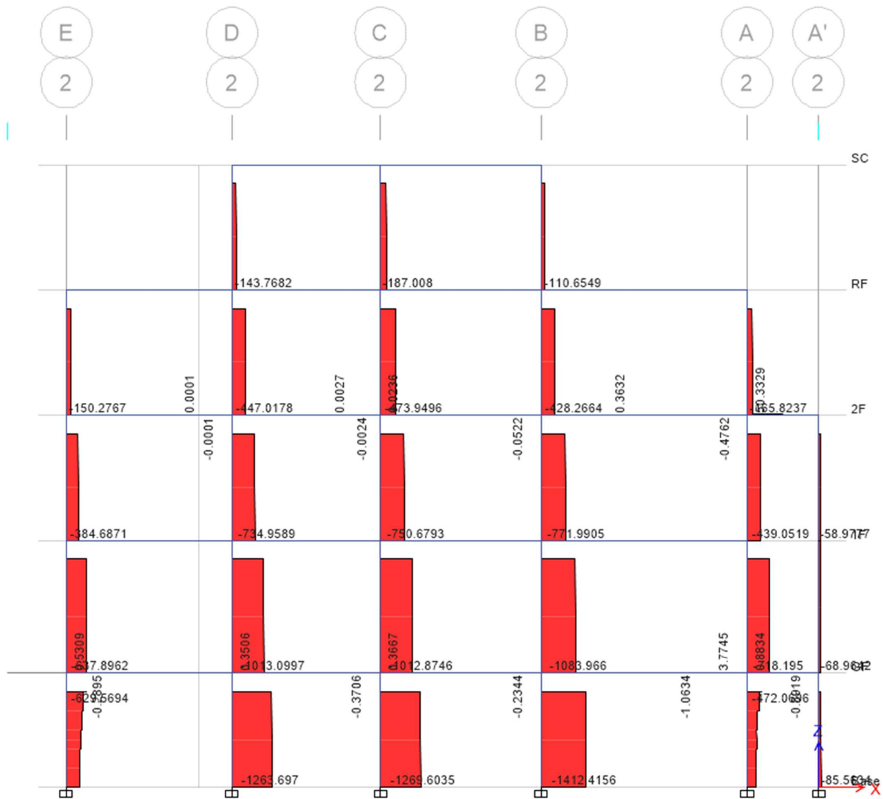
Fig: AFD for Frame 2-2 (1.5DL+LL)
